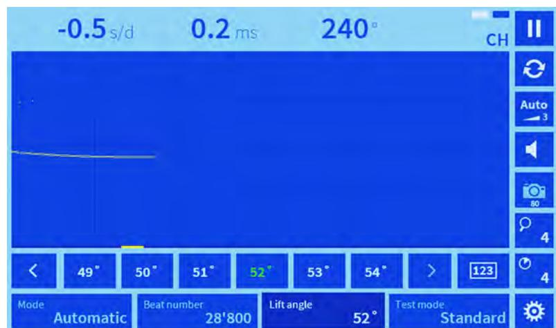
Fig. 17: Selecting a lift angle manually
