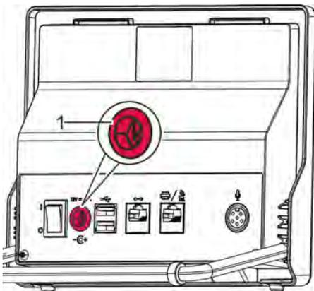
2. ➤ Insert the power supply unit adapter into the mains connection (Fig. 10/1).
