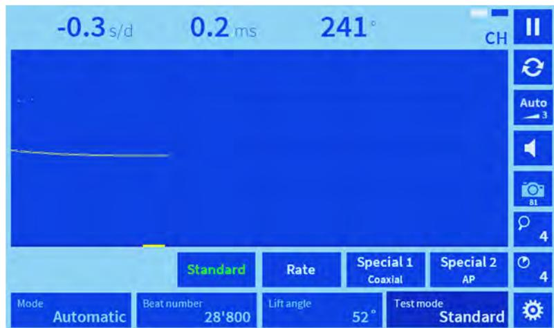
Fig. 19: Selecting test mode
