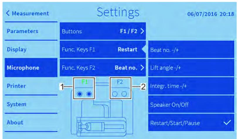
Fig. 36: Assigning functions
