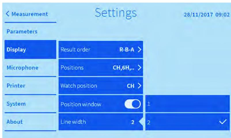
Fig. 34: Determination of line thickness (only in Diagram display mode)
