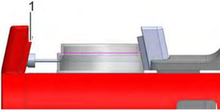
Fig. 24: Clockwork clamped in cup
