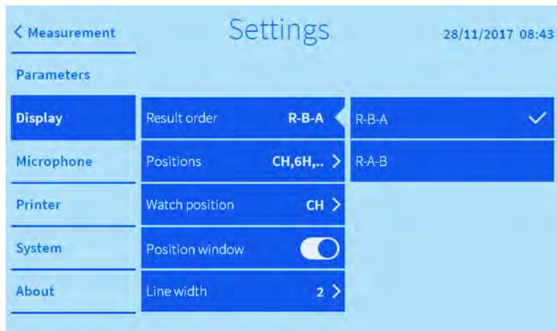
Fig. 30: Setting the display sequence of the current measured values
