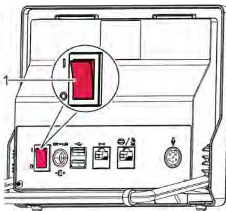
Fig. 13: Switching on the Watch Expert
