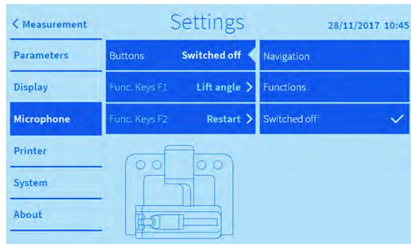
Fig. 37: Switching off the microphone buttons
