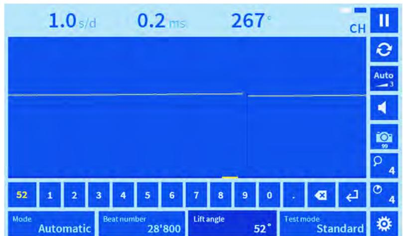
Fig. 18: Entering a lift angle manually
