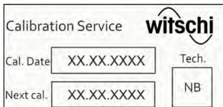
The calibration instruction on the underside of the device shows when the device needs to be recalibrated. To ensure reliable measuring results, we recommend observing the proposed date for the next calibration.
